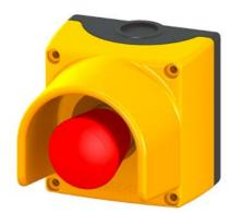
ENCLOSURE FOR COMMAND DEVICES, 22MM, ROUND, ENCLOSURE MATERIAL PLASTIC, YELLOW TOP PART, WITH PROTECTIVE COLLAR, 1 COMMAND POSITION, A=EMER.-STOP MUSHROOM PUSHBUTTON RED, 40MM, ROT.-TO-UNLATCH MECHANISM, 1NC, 1NC, SCREW TERMINAL, FLOOR MOUNTING, TOP AND BOTTOM 1 X M20 EACH !!! Phased-out product SIRIUS ACT 3SU1 is s Preferred successor type is >>3SU1801-0NB00-2AC2<<
