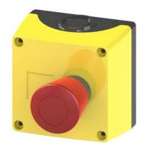
Enclosure for command devices, 22 mm, round, enclosure material plastic, enclosure top part yellow, 1 control point, A=Emergency stop mushroom pushbutton red, 40 mm, rotate-to-unlatch, 1 NC, 1 NC, screw terminal, floor mounting, top and bottom 1 x M20 each ! Phased-out product! Successor is SIRIUS ACT 3SU1
