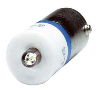
ACCESSORY / SPARE PART ROUND, 22MM/SQUARE, 26X26MM: LED SUPER-BRIGHT LAMPS, BASE BA 9S BULB DIAMETER 10MM RATED VOLTAGE 130V AC-90V DC OPERATIONAL CURRENT MAX. 15 MA GREEN
