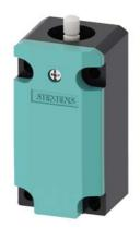
Basic switch for position switch 3SE51 Metal enclosure, according to EN 50041 1x (M20x 1.5) 1 NO/1 NC slow-action contacts without actuator head
