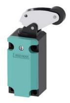
Position switch Metal enclosure 40 mm according to EN 50041 Device connection 1x (M20 x 1.5) 1 NO/1 NC quick action contacts Angular roller lever, metal lever and plastic roller 22 mm
