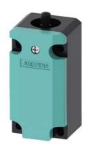
Basic switch with increased corrosion protection for position switch Metal enclosure, according to EN 50041 Device connection 1 x (M20 x 1.5) 1 NO/2 NC quick action contacts without actuator head
