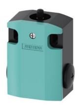
Position switch Basic switch Metal, 56 mm Increased corrosion protection 1 NO/2 NC quick action contacts functional at -40 °C Shock and vibration test according to EN 61373, Category 1B
