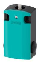
Basic switch for position switch 3SE5162 Metal enclosure XL, 56 mm wide Device connection  $3x(M20\ x\ 1.5)$  IP66/IP67 2 x (1 NO/2 NC) Slow-action contacts without actuator head
