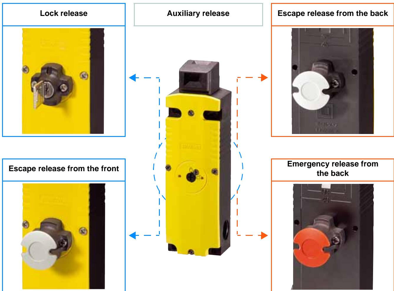
■ Personnel working inside the hazard zone can use the **escape release** feature to manually release the tumbler without tools so that they can exit the hazard area. An intentional act (in this case pulling the gray actuator) is required to release the locking mechanism and restore the normal operating state.
