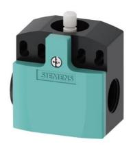
position switch plastic 50 mm increased corrosion protection device connection 2x (M20x 1.5) 1 NO/1 NC integrated (not replaceable) quickaction contacts, rounded plunger, functional at -40 °C shock and vibration test according to EN 61373, category 1B
