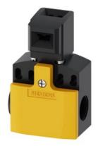
Safety position switch with separate actuator Plastic enclosure, 50 mm Device connection 2x (M20x 1.5) Slow-action contacts 1 NO+2 NC 5 directions of approaches The matching separate actuator 3SE5000-0AV0. must be ordered separately
