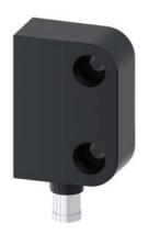
magnetically-operated switch contact block, rectangular small 26 x 36 mm, for door hinge left, contacts: safety contacts 2 NC, signaling contact 1 NC (31-32), with 8 mm latching connection connector 6-pole, without LED, the matching solenoid 3SE6714-3CA or offset by  $90^\circ$  3SE6724-3CA
