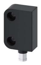
Magnet switch Switching element, rectangular small 26 x 36 mm, for door hinge on the right, Contact elements: Safety contacts 1 NO+1 NC Signaling contacts 1 NC with 8 mm latching connection Connector 6-pole, without LED the matching solenoid 3SE6714-3CA or offset by 90° 3SE6724-3CA
