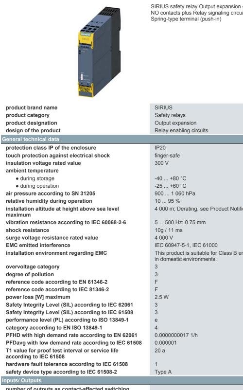
SIRIUS safety relay Output expansion 4RO with relay enabling circuits 4 NO contacts plus Relay signaling circuit 1 NC contact Us = 24 V DC
