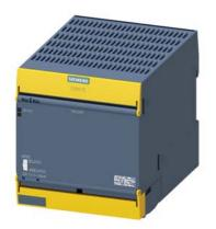
SIRIUS safety relay Output expansion 3RO Power, with Relay enabling circuits 3 NO contacts plus Relay signaling circuit 1 NC contact Us = 24 V DC Spring-type terminal (push-in)
