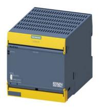
SIRIUS safety relay Output expansion 3RO Power, with Relay enabling circuits 3 NO contacts plus Relay signaling circuit 1 NC contact Us = 24 V DC screw terminal
