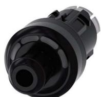
ID key-operated switch, 22 mm, round, plastic, black, RFID, 4 switch positions O-I-II-III, operating angle  $3x45^{\circ}$ , without ID key, Key removal in O+I+II+III
