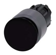
Mushroom pushbutton, 22 mm, round, plastic with metal front ring, black, 30 mm, latching, Pull-to-unlatch mechanism
