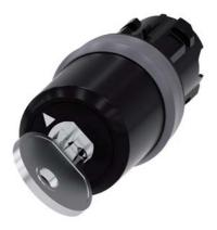
key-operated switch Siemens, 22 mm, round, plastic with metal front ring, lock number SSG10, with 2 keys, 2 switch positions O-I, latching, actuating angle 90°, 10:30h/13:30h, key removal O+I
