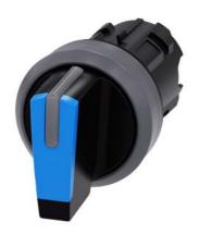
Selector switch, illuminable, 22 mm, round, plastic with metal front ring, blue, selector switch, short, 3 switch positions I>O<II, momentary contact type, actuating angle 2x45°, 10:30h/12h/13:30h
