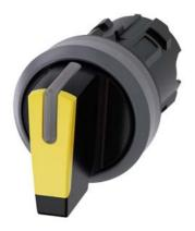
Selector switch, illuminable, 22 mm, round, plastic with metal front ring, yellow, selector switch, short, 3 switch positions I>O<II, momentary contact on the left, latching on the right, actuating angle  $2x45^{\circ}$ , 10:30h/12h/13:30h
