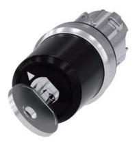
key-operated switch Siemens, 22 mm, round, metal, shiny, lock number SSG10, with 2 keys, 2 switch positions O-I, latching, actuating angle 90°, 10:30h/13:30h, key removal O+I
