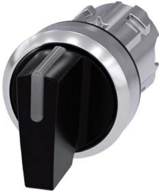
Illuminable selector switch, 22 mm, round, metal shiny, black, Selector switch short, 3 switch positions I-O-II, latching, actuating angle 2x45°, 10:30h/12h/13:30h
