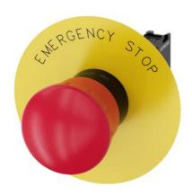
EMERGENCY STOP mushroom pushbutton, 22 mm, round, plastic, red, 40 mm, positive latching, acc. to EN ISO 13850, rotate-to-unlatch, with yellow backing plate, inscription: EMERGENCY STOP, with holder, 1 NC, screw
