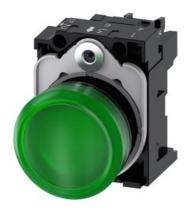
Indicator lights, 22 mm, round, plastic, green, lens, smooth, with holder, LED module with integrated LED 110 V AC, screw terminal
