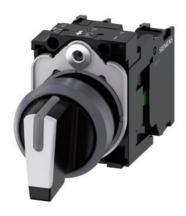
Selector switch, illuminable, 22 mm, round, plastic with metal front ring, white, selector switch, short, 3 switch positions I>O<II, momentary contact type, actuating angle 2x45°, 10:30h/12h/13:30h, with holder, 1 NO, 1 NO, screw terminal
