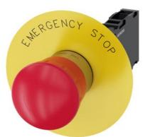
EMERGENCY STOP mushroom pushbutton, 22 mm, round, metal, shiny, red, 40 mm, positive latching, acc. to EN ISO 13850, rotate-to-unlatch, with yellow backing plate, inscription: EMERGENCY STOP, with holder, 1 NO+1 NC, screw terminal
