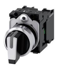
Selector switch, illuminable, 22 mm, round, metal, shiny, white, selector switch, short, 3 switch positions I>O<II, momentary contact type, actuating angle 2x45°, 10:30h/12h/13:30h, with holder, 1 NO, 1 NO, screw terminal
