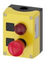
Enclosure for command devices, 22 mm, round, Enclosure material plastic, Enclosure top part yellow, 2 control points plastic, B=Indicator light red, LED 24 V, screw terminal, label without inscription, A=Emergency stop 40 mm rotate-to-unlatch, label without inscription, 1 NO, 1 NC, 1 NC, screw terminal, floor mounting, 1xM20 each on top and bottom, Labels enclosed
