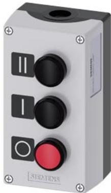
Enclosure for command devices, 22 mm, round, Enclosure material plastic, enclosure top part gray, 3 control points plastic, C=Pushbutton black, Label: II, 1 NO, screw terminal, B=Pushbutton black, Label: I, 1 NO, screw terminal, A=Pushbutton red, label: O, 1 NC, screw terminal, floor mounting, 1xM20 each on top and bottom, Labels enclosed
