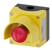
Enclosure for command devices, 22 mm, round, Enclosure material metal, Enclosure top part yellow, with protective collar, 1 control point metal, A=EMERGENCY STOP mushroom pushbutton red, 40 mm, rotate-to-unlatch, 1 NC, 1 NC, screw terminal, floor mounting, 1xM20 each on top and bottom
