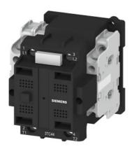
Contactor, Size 2, 2-pole, DC-3 and 5, 32 A Auxiliary contacts 11 (1NO + 1NC) 2x solid-state compatible auxiliary contact AC operation 120 V AC 50/60 Hz Special-purpose device
