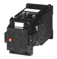
Contactor, Size 2, 2-pole, DC-3 and 5, 32 A Auxiliary contacts 22 (2 NO + 2 NC) 125V DC DC operation
