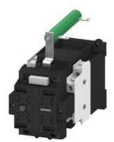
Contactor, Size 2, 2-pole, for railway applications DC-3 and 5, 7.5 A at 750 V 24 V DC Auxiliary contacts 21 (2NO+1NC) with varistor and series resistor Operating range 0.7...1.25xUS Operating range 0.7...1.25xUS
