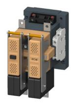
Contactor, Size 4, 2-pole, DC-3 and 5, 75 A Auxiliary switch 22 (2 NO + 2 NC) 240 V AC 50 Hz/288 V AC 60 Hz AC operation
