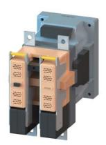
Contactor, Size 8, 2-pole, DC-3 and 5, 220 A Auxiliary switch 22 (2 NO + 2 NC) 230 V DC DC operation
