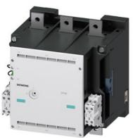
Contactor, Size 14, 3-pole, AC-3, 335kW, 400/380 V (690 V) Auxiliary switch 44 (4NO+4NC) AC operation 110...132 V AC 50/60 Hz
