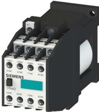
Contactor relay, 62E, DIN EN 50011, 6 NO + 2 NC, screw terminal DC operation 24 V DC
