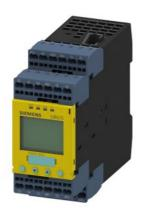
SIRIUS safety relay Safety-oriented Speed monitoring 24 V DC, 45 mm overall width Spring-type terminal EC instantaneous: 2 NO EC delayed: 0 SC: 2 electrical Auto-start/manual start Basic device Maximum achievable PL according to EN 13849-1: e Maximum achievable SIL according to IEC 61508: 3
