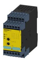
SIRIUS safety relay safety-oriented Standstill monitoring 24 V DC, 45 mm screw terminal EC instantaneous: 3 NO + 1 NC EC delayed: 0 SC: 3 Autostart Basic unit max. error category EN 954-1: 4 Maximum achievable PL according to EN 13849-1: Maximum achievable SIL according to IEC 61508: 3
