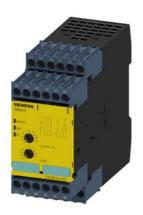
SIRIUS safety relay safety-oriented Standstill monitoring 230 V AC, 45 mm screw terminal EC instantaneous: 3 NO + 1 NC EC delayed: 0 SC: 3 Autostart Basic unit max. error category EN 954-1: 4 Maximum achievable PL according to EN 13849-1: Maximum achievable SIL according to IEC 61508: 3
