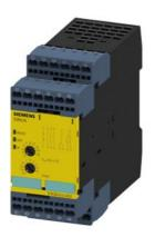
SIRIUS safety relay safety-oriented Standstill monitoring 400 V AC, 45 mm Spring-type terminal EC instantaneous: 3 NO + 1 NC EC delayed: 0 SC: 3 Auto-start Basic unit max. error category EN 954-1: 4 Maximum achievable PL according to EN 13849-1: Maximum achievable SIL according to IEC 61508: 3
