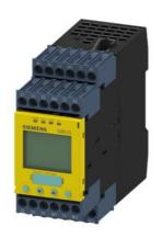
SIRIUS safety relay Safety-oriented Speed monitoring 24 V DC, 45 mm overall width Screw terminal EC instantaneous: 2 NO EC delayed: 0 SC: 2 electrical NAMUR version Auto-start/manual start Basic device Maximum achievable PL according to EN 13849-1: e Maximum achievable SIL according to IEC 61508: 3
