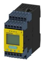
SIRIUS safety relay Safety-oriented Speed monitoring 110-240 V AC/DC, 45 mm overall width Screw terminal EC instantaneous: 2 NO EC delayed: 0 SC: 2 electrical Auto-start/manual start Basic device Maximum achievable PL according to EN 13849-1: e Maximum achievable SIL according to IEC 61508: 3
