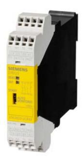
SIRIUS SAFETY RELAY WITH RELAY ENABLING CIRCUITS, 24 V AC/DC, 22.5MM, SPRING-LOADED TERMINAL, BASIC UNIT, AUTO START, MONITORED START INSTANTANEOUS: 3NO, DELAYED: 0NO, SIGNALING CIRCUIT: 1NC, MAX. ERR. CAT. EN954-1: 4 SIL: 3,
