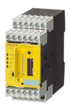
!!! Phased-out product !!! The successor product series is 3SK2 (see FAQ 109741483) SIRIUS safety relay with relay enabling circuits (EC) 24 V DC, 45 mm screw terminal EC instantaneous: 2 NO EC delayed: 2 SC: 4 Switch with 8 functions Basic device Maximum achievable PL according to EN 13849-1: Maximum achievable SIL according to IEC 61508: 3
