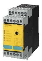
SIRIUS safety relay with relay enabling circuits (EC) 115 V AC, 45 mm overall width Screw terminal EC instantaneous: 2 NO EC delayed: 2NO, 0.5...30 s SC: 1NC monitored start Basic device Maximum achieved SIL: 3/2, PL: e/d
