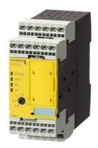
SIRIUS safety relay with relay enabling circuits (EC) 24 V DC, 45 mm overall width Spring-type terminal EC instantaneous: 2 NO EC delayed: 2NO, 0.05...3 s SC: 1NC monitored start Basic device Maximum achieved SIL: 3/2, PL: e/d
