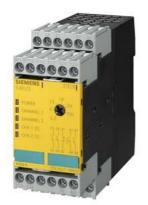
SIRIUS safety relay with relay enabling circuits (EC) 115 V AC, 45 mm overall width Screw terminal EC instantaneous: 2 NO EC delayed: 2NO, 0.5...30 s SC: 1NC AUTOSTART Basic device Maximum achieved SIL: 3/2, PL: e/d
