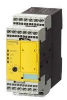
SIRIUS safety relay with relay enabling circuits (EC) 24 V DC, 45 mm overall width Spring-type terminal EC instantaneous: 2 NO EC delayed: 2NO, 0.05...3 s SC: 1NC AUTOSTART Basic device Maximum achieved SIL: 3/2, PL: e/d
